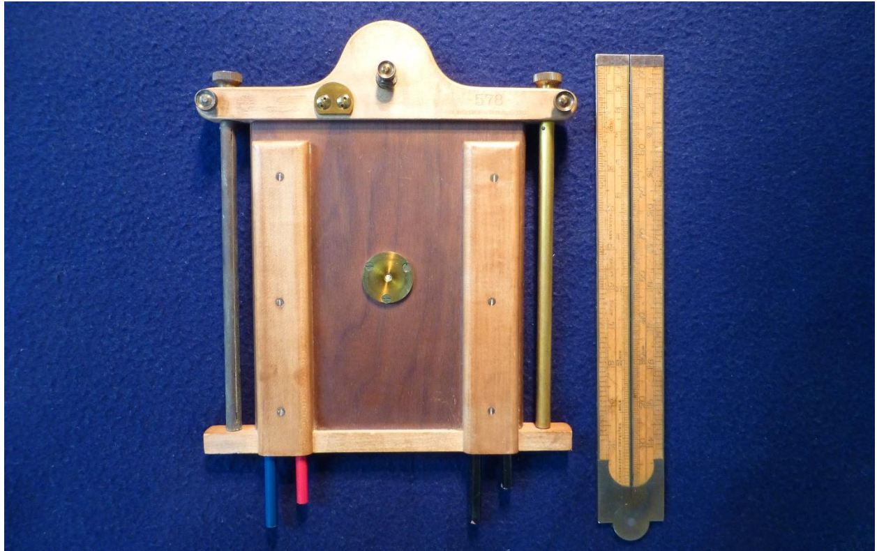
The back of the board, showing the compass lock at top, the threaded fitting for the wrist strap at center, and the pencil tubes for one blue, one red and two black pencils.
